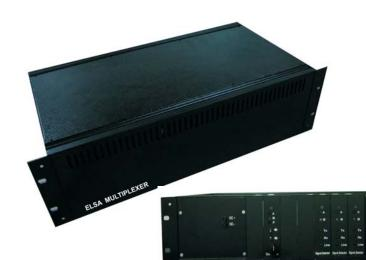
ELSA Multiplexer EM-14L is designed using two processors and works redundantly. This system can transmit/receive data from two RS-232 input serial ports to one RS-232 output serial port. The input priority can be set-up to avoid data collision. Casing is designed using 19" standard and 3U height to be placed in 19" standard rack.
