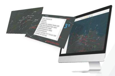
Elsa radar/ADS-B display is an application software for visualizing ADS-B / radar data. Data that is transmitted by multicast over a LAN (network) containing aircraft position, latitude, longitude, altitude, speed and aircraft-ID will be received and processed by the application so that the data is displayed visually and in real-time.
